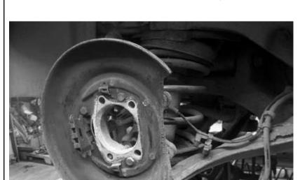
For a broken handbrake stop - with the hand brake shoe bracket you don't have to replace the entire brake shoe attaching plate.
