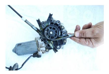
Mount the top cable around the top corner wheel and fit the cable in the window slider. Push slider down the rail to compress the spring by using a mole to grip the rail. Some of the wheels have a small "V" in them to feed the cable past the guide. Either file a small "V" in the wheel or bend the small lug back. Remember to bend the lug to its original position to keep the cable in place.
