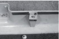
\* Remove all plastic clips and replace with clips included in the kit both top and bottom
